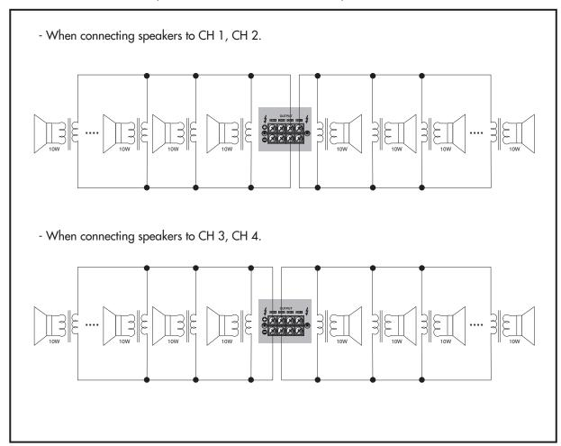
\* Caution: 1. Make sure that the total impedance does not equal or less than the rated impedance.
