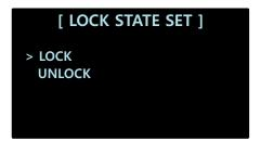
In LOCK PANEL, you can LOCK or UNLOCK the functions controlled from the front of the device. If you set the device to LOCK, the system will redirect you to the initial OLED screen, and you will not be able to use the buttons at the front of the device. To UNLOCK the device, press down the SELECT/ENTER (ENCODER) dial at the front, then type the LOCK/UNLOCK password. The initial password is 0000.
