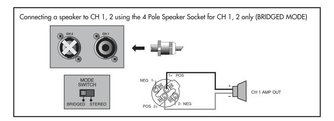
\*\* Caution: When installing the system, ensure that the total impedance of the speaker does not fall below the regulated impedance (4 $\Omega$ , 8 $\Omega$ ) under all circumstances. Otherwise, it may lead to overloading and cause the system to fail.
