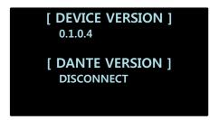
In VERSION, you can check the firmware version, DANTE NETWORK version of the current device. The screen will display the firmware version of the device at all times. However, it will display the DANTE NETWORK version only when DANTE is connected to the device.
