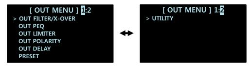
The OUT MENU features multiple items including OUT FILTER/X-OVER, OUT PEQ, OUT LIMITER, OUT POLARITY, OUT DELAY as well as PRESET and UTILITY. PRESET, UTILITY items are also available in the IN MENU.
