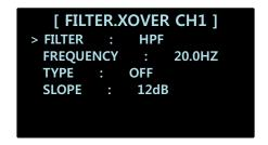
In FILTER/X-OVER settings, you can set up each channel differently.
