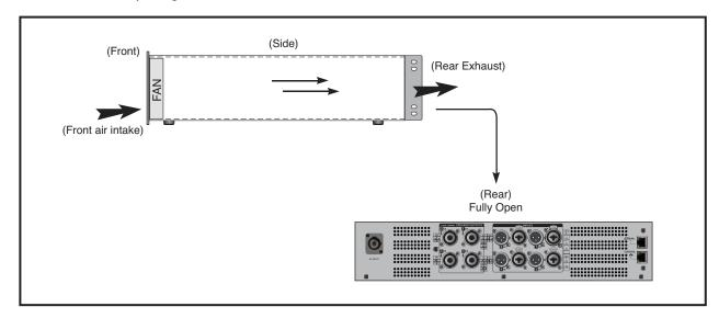
2. When using power amplifier, please install the unit where there is no airflow block to the heat sink.
