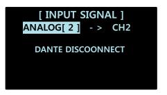
In SOURCE settings, you can distribute the audio signal received through the XLR INPUT/LINK terminal at the back of the device or through the network and the DANTE Digital Audio PORT to the output channel (speaker connection terminal) you want to use. Initial configuration: ANALOG[1]->CH1, ANALOG[2]->CH2, ANALOG[3]->CH3, ANALOG[4]->CH4. You can select from 8 SOURCES, including ANALOG [1]-[4], DANTE [RX0]-[RX3], etc.
