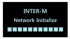
This initial screen appears when the power cable is connected to the set and the DSP begins to boot up. If indicates that the device is currently booting up. Boot-time is approximately 10 seconds.
