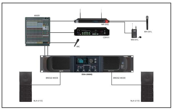
• How to connect a PE12 and NLA-5/15S with BRIDGED MODE
