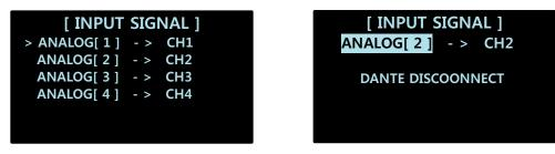
In SOURCE settings, you can distribute the audio signal received through the XLR INPUT/LINK terminal at the back of the device or through the network and the DANTE Digital Audio PORT to the output channel (speaker connection terminal) you want to use. Initial configuration: ANALOG[1]->CH1, ANALOG[2]->CH2, ANALOG[3]->CH3, ANALOG[4]->CH4. You can select from 8 SOURCES, including ANALOG [1]-[4], DANTE [RX0]-[RX3], etc.
