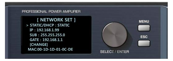
In NETWORK SETUP, you can check the NETWORK specifications of the current device.
