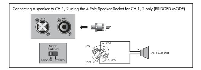
\* Caution: When installing the system, ensure that the total impedance of the speaker does not fall below the regulated impedance ( $4\Omega$ ,  $8\Omega$ ) under all circumstances. Otherwise, it may lead to overloading and cause the system to fail.
