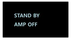
This screen indicates that the power cable has been connected and the power switch remains OFF, but the device has completed its boot-up protocol. If you turn the switch ON when the system is displaying this screen, power will be supplied and the OLED control screen will appear.
