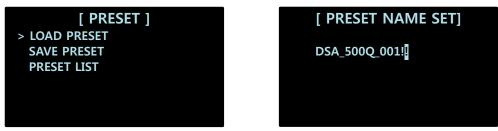
PRESET settings offers Load preset, Save preset, and Preset List functions. Instructions for PRESET settings are identical to the instructions for PRESET settings from the IN MENU. For more detailed setting instructions, please refer to section 4. 5 PRESET SETTING on page 17 of this manual.
