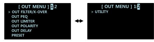
The OUT MENU features multiple items including OUT FILTER/X-OVER, OUT PEQ, OUT LIMITER, OUT POLARITY, OUT DELAY as well as PRESET and UTILITY. PRESET, UTILITY items are also available in the IN MENU.
