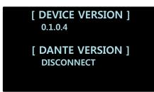
In VERSION, you can check the firmware version, DANTE NETWORK version of the current device. The screen will display the firmware version of the device at all times. However, it will display the DANTE NETWORK version only when DANTE is connected to the device.
