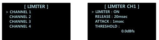
In LIMITER settings, you can set up each channel differently.
