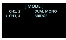
In MODE settings, you can select 5 different modes: DUAL MONO, STEREO, BI-AMP 1, BI-AMP 2, and BRIDGE. Initially, CH1, 2, 3, 4 are all set to DUAL MONO.
