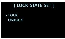
In LOCK PANEL, you can LOCK or UNLOCK the functions controlled from the front of the device.
