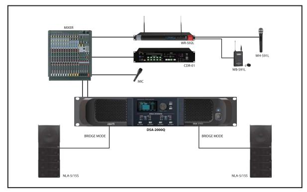
• How to connect an NLA-5/15S with BRIDGED MODE (DSA-2000Q)
