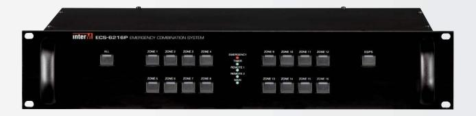
The ECS-6216P is the main primary output zone module that allows the addition of 16 output zones to the system 6000. Up to 160 outputs zone capacity is possible with the addition of up to 9 additional ECS-6216S. Each unit also offer an addition of 16CH GPI sensor input for messaging, event and scenario triggering.
