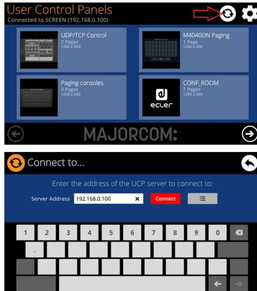
This page allows deciding the UCP server the unit will connect to as a client. The UCP server may be a computer, a matrix (Yes, it has an embedded UCP server in its engine!) another EW-SCREEN / W-SCREEN unit or even the same EW-SCREEN unit. In any case, the UCP server shall host and run a Majorcom NetManager project that includes a series of UCPs which can be remotely managed by any UCP client.
