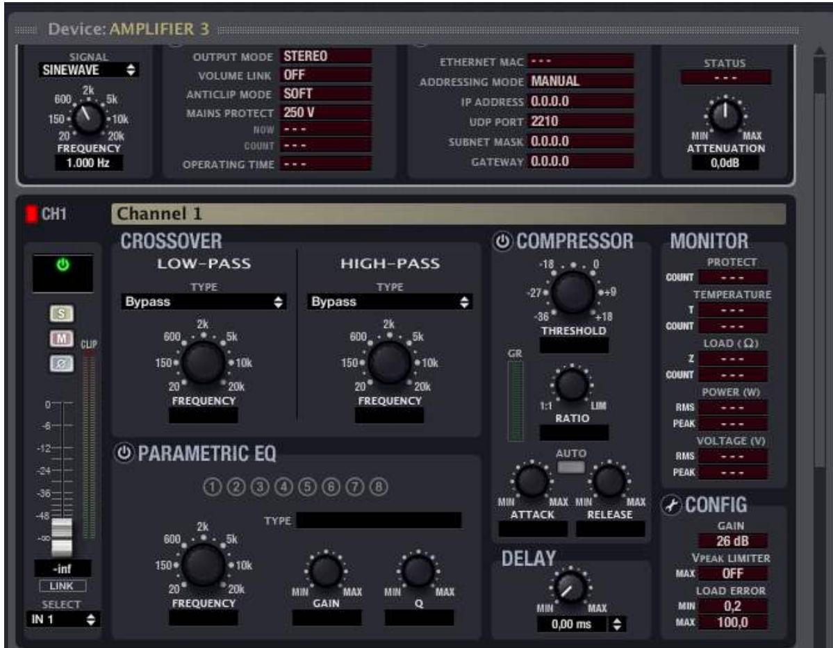
Device window for NPA series device
