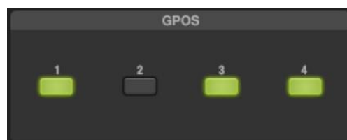
In the picture the GPO 1, 3, and 4 are active and GPO2 is inactive
