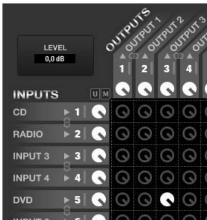
MUTE OFF for input 5 – output 3 (send enabled)
