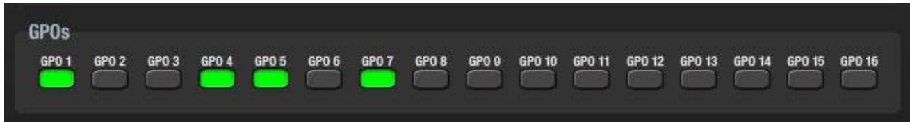
In the picture the GPO 1, 4, 5 and 7 are active and the rest of them are inactive
