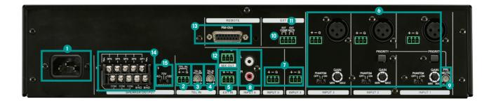
AC INPUT PRIORITY CONTROL VOLUME (PRIORITY MUTE) TEL IN INPUT TERMINAL **(D)** EXTERNAL CHIME (EXT CHIME) SWITCH TERMINAL TEL IN VOLUME CONTROLLER EXTERNAL MUTE SWITCH TERMINAL S TEL IN PRIORITY CONTROL VOLUME (TEL IN MUTE) 20 MIX OUTPUT (MIX OUT) TERMINAL EXTERNAL INPUT (EXT IN) TERMINAL RM-05A CONNECTION TERMINAL INPUT 1~3 (MIC/LINE) SPEAKER OUTPUT TERMINAL INPUT 4~5 (LINE) IMPEDANCE SELECTION SWITCH
