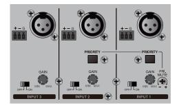
(1) PHANTOM Switch: If you want to use a condenser microphone, turn this switch on to provide DC 24V PHANTOM power.
