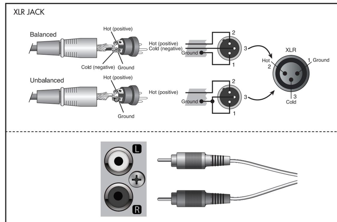
Connect a stereo output source device to the RCA connectors of the INPUT 2. (Unbalanced, 0dBV/1Vrms)
