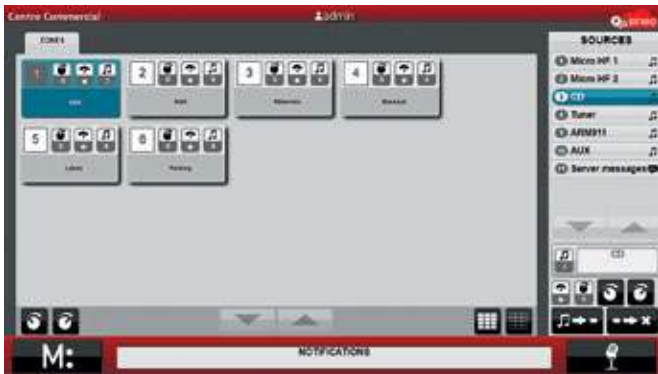
Routing source to any zone, manage input levels and volumes zones
