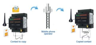
Point-to-point application between 2 SMS-112 transmitters (+ SIM cards). When a contact state changes on SMS-112 #1, it sends a command to SMS-112 #2 to close one of its outputs.
