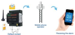
Sending an alarm by SMS, Mail or Voicemail in the event of an electrical dry contact tripping when the threshold of an analog input is exceeded or if the power supply is cut.
