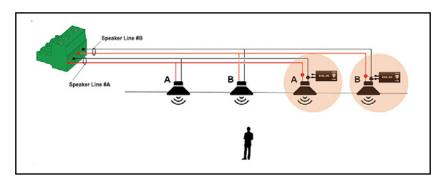
The EOL-20 must be connected at the end of the line and on each speaker line. The two wires have no polarity and can therefore be connected in either direction.
