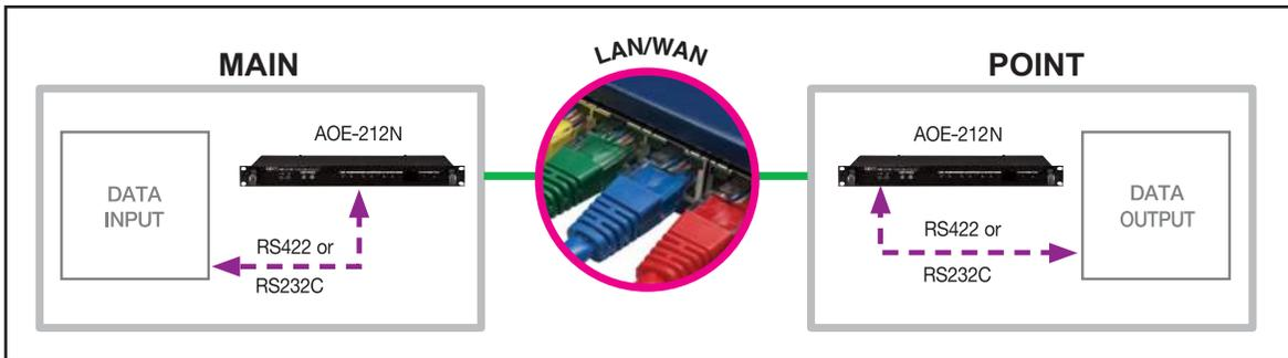
RS-232C communication: No. 1 pin (Rx), No. 3 pin (Tx), No. 5 pin (GND)
