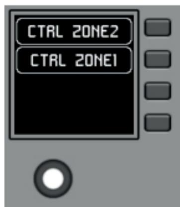
In the previous example it can be seen that there are two possible individual panels as options for the MULTI panel to take its role: CTRL ZONE1 and CTRL ZONE2. By means of K1 and K2, in this case, it is possible to select one or the other. Example by selecting the individual panel CTRL ZONE2 (key K2) :
