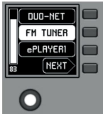
When acting on the K5 rotary control, aiming at modifying the volume to which it points, a different screen is temporarily shown, returning a few seconds to the previous or main screen. Example :
