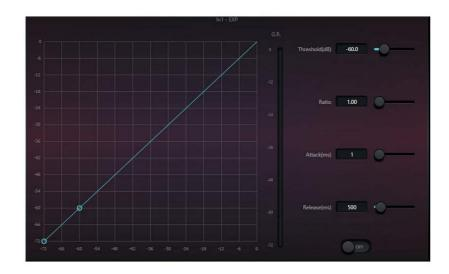
Threshold : The expander engages when the signal is below this threshold.
