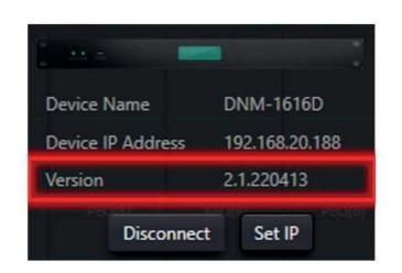
2. Send the Factory Reset hex command via UDP to port 6001 of the DNM unit using a UDP sender app such as Packet Sender or Hercules. The Factory Reset code can be found on a sticker affixed to the DNM. The code can be identified as starting with 'A5'.
