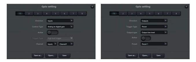
All DNM units above 8x8 channels include 8 GPIO interfaces. The "GPIO Setting" dialog allows for the configuration of this I/O.
