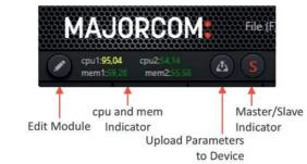
Below the main software logo is the Edit Module mode button with a pencil icon. Pressing this button enters to module edit mode where individual DSP Modules can be added or removed from channels.
