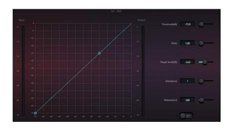
Threshold: When the signal level is lower than the threshold, the input-to-output ratio is 1:1. When the signal level is higher than the threshold, the input-to-output ratio changes according to the ratio control settings. The threshold will typically be set just above the noise floor. This assures that the noise floor itself will not trigger the AGC, but any signal above that will.
