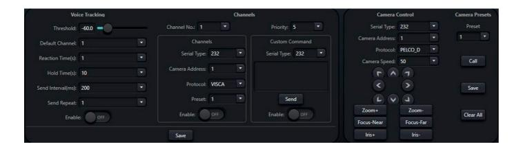
The Camera Tracking tab is split into two distinct functional categories. The first two sections are tied together to configure Automatic Voice Tracking Cameral Control. The two sections to the furthest right of the panel function as live, Manual Camera Control.
