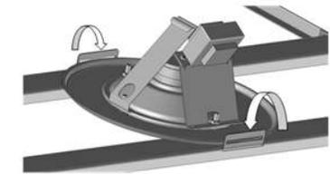
The whole product is installed as a standard false ceiling tile.
