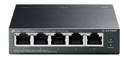
SWITCH POE 5P is a 5 10/100/1000Mbps ports unmanaged switch that requires no configuration and provides 4 PoE (Power over Ethernet) ports. It can automatically detect and supply power with all IEEE 802.3af compliant Powered Devices (PDs). In this situation, the electrical power is transmitted along with data in one single cable allowing you to expand your network to where there are no power lines or outlets, where you wish to fix devices such as APs, IP Cameras or IP Phones, etc.
